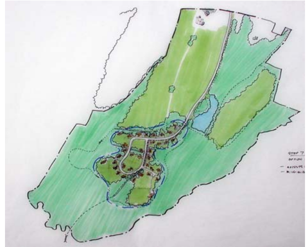
*Final approved subdivision plan with the limits of disturbance for developed area and conservation easement area
